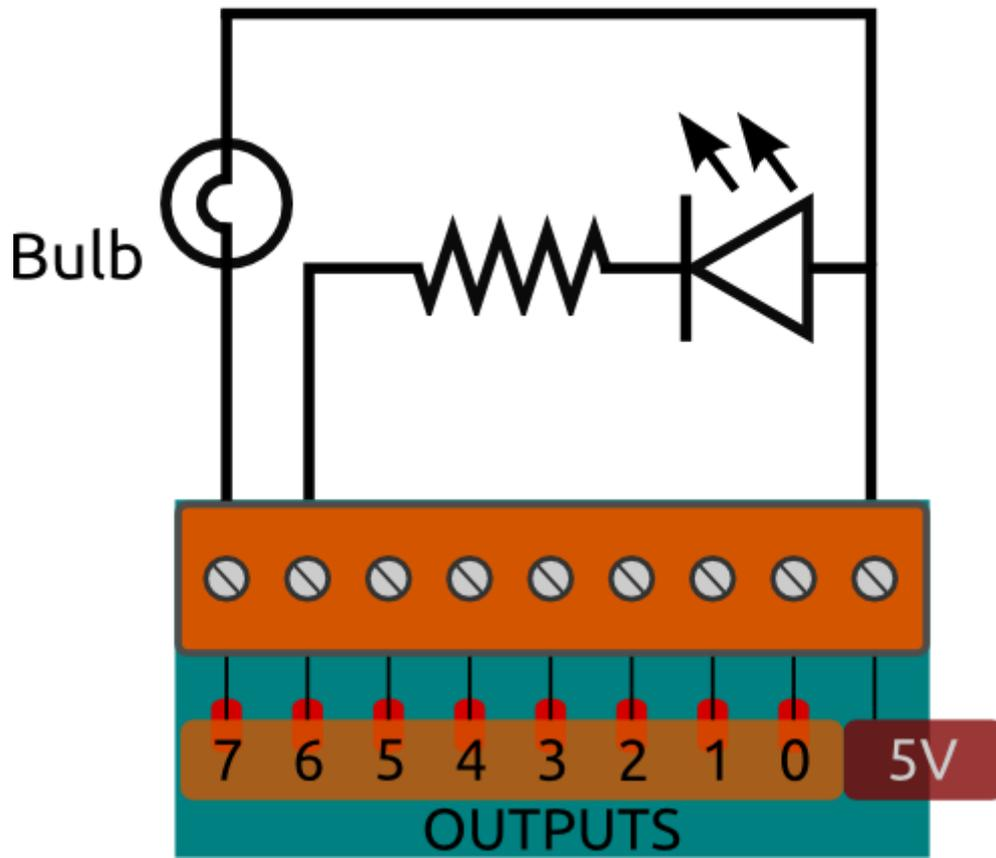
example connection for bulb and LED
