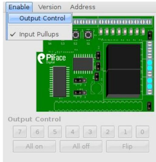
Toggle output pin 0 on by clicking on the '0' button. The first Relay on PiFace™ Digital will click as it turns on and the corresponding LED will illuminate (if the jumpers are in their default settings). Notice the graphic on screen updates to show the state of the LED, the contacts on the relay and the first output pin.
