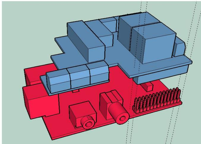
Original PiFace™ Digital fitting onto Raspberry Pi® model B
