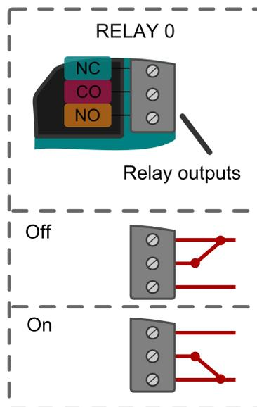
The relays may be disabled by removing the appropriate jumper (JP5 and JP6) as detailed in *Jumper settings*.
